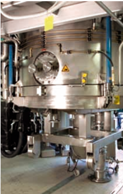
Hastelloy reactor used for pharmaceutical active substances
