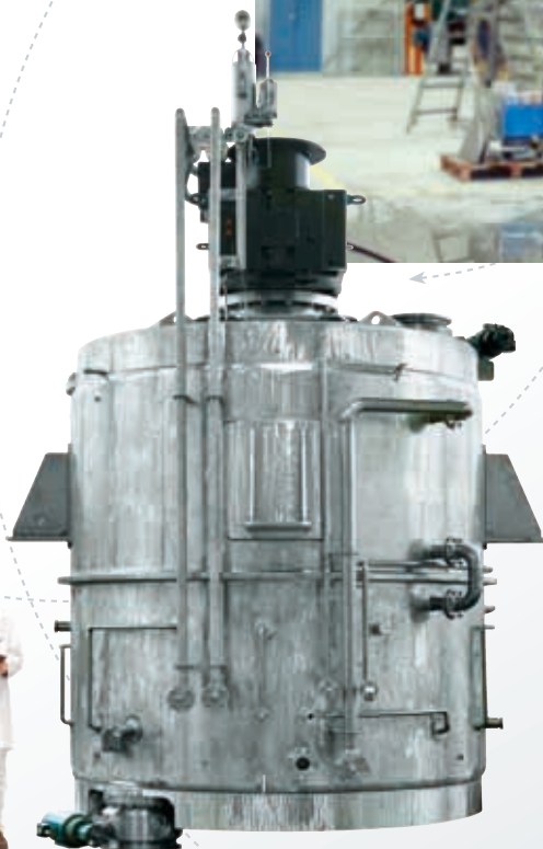
Mixer dryer reactor used for 14 m³ batches
