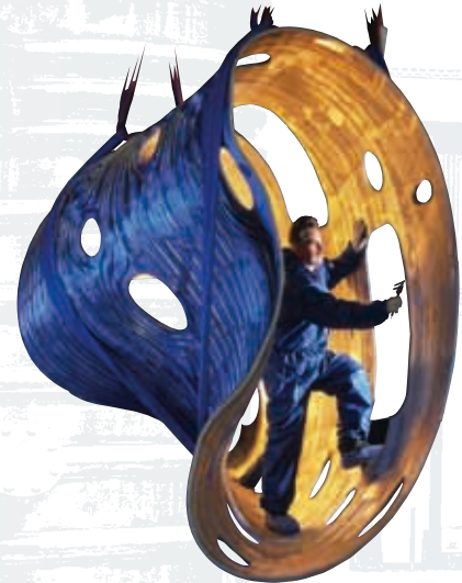
Reactor vessel cut by Clever-Cut®, Max-Planck-Institut für Plasmaphysik
