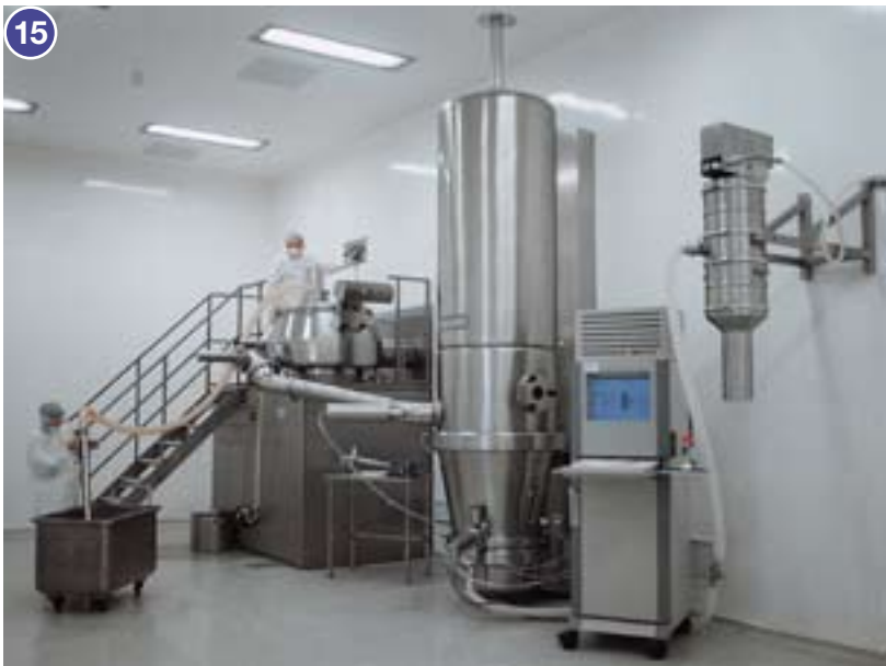
Fig. 15: Vacuum Conveyor for the automatic discharging of a fluidized bed dryer. Product delivery through an submer-sion tube into IBCs.
