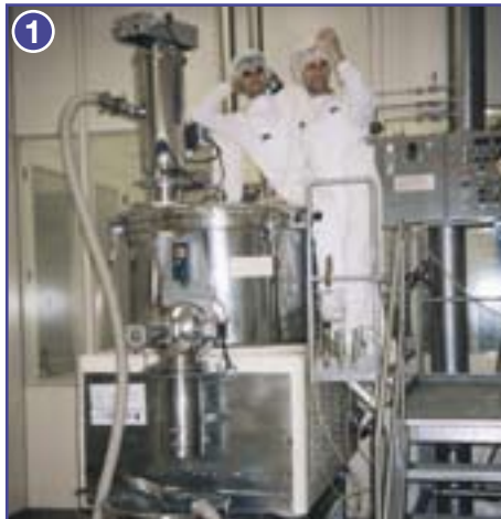
Fig. 1: PPC250 installation to transfer Paracetamol powder from a drum into a mixer.
