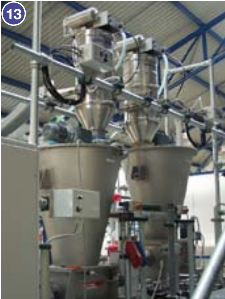
Fig. 1: Filling of a mixing and a reaction vessel with flame soot, manganese dioxide and calcium carbonate. Continuously working tandem Vacuum Conveyor.
