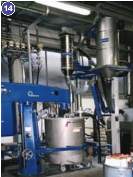
Fig. 9: Filling of toner powder into cartridges with a Vacuum Conveyor VR315.
